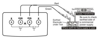
Risk: Be careful of electric shock when using commercial electric system earth method for test.
